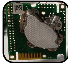
Ambient CO 2 Sensor
